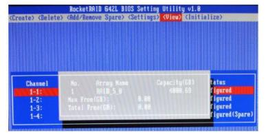
RAID Array – This option will display information about each RAID array hosted by the HBA. Highlight the target device and press Enter to view details about the configuration.
