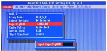
Note: Multiple arrays can be created using the same set of hard disk drives. The Capacity option allows you to set aside disk space that be used to create another array, set as a spare disk, or partitioned to act as a single disk (by the operating system).
